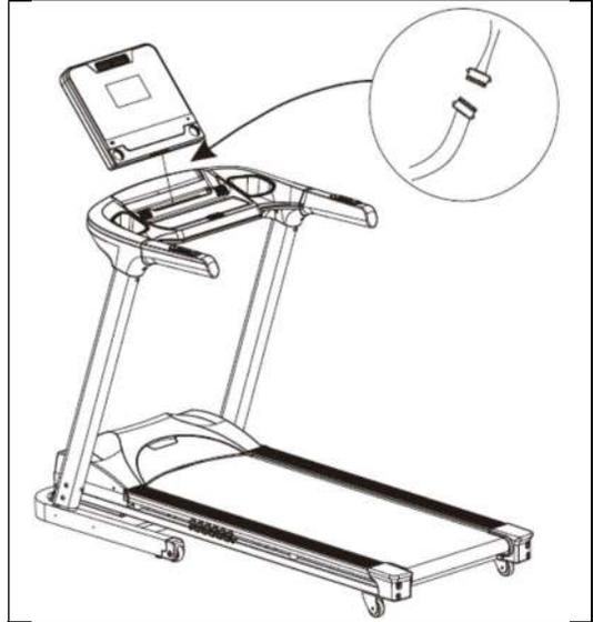
5. Remove the 3 x M6\*15 screws from the back of the console. Make sure not to discard them. Place the console inside the console base. Ensure not to pinch or crush the signal wires. Use the 3 x M6\*15 screws to fasten the console back onto the console base.
